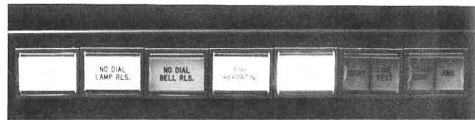
These indicators at the base of the Security Alarm System console pinpoint the particular report for the attendant on duty, while the display shows the location reporting. The indicators also serve as release keys, since the console automatically locks-in the station signaling an alarm.
