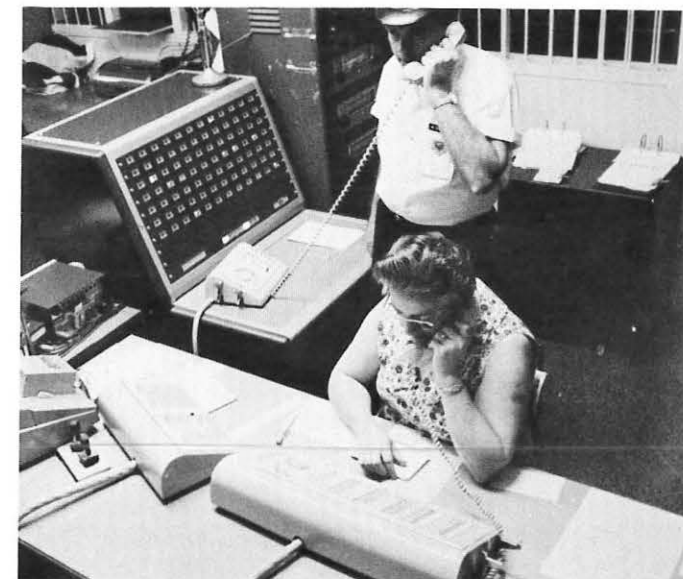
This is the communications center of the Maryland Correctional Institution. The guard at the Security Alarm System console talks with a reporting security guard at one of the phone locations. The console, heart of the Institution's new communications system, has visual and audio indicators to signal alarm conditions. Lights in the console's miniature displays indicate phone stations reporting as well as phones in use. At left (resembling an adding machine) is the print-out device which automatically records date, time and station number reporting in via Security Alarm System. In the foreground, an attendant handles the regular phone traffic using a modern desk-top console and direct station selection equipment.
